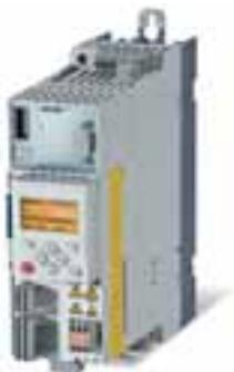
The 8400 StateLine has been designed specifically for drive controls with or without speed feedback and is used wherever networking via bus systems is required. Furthermore, integrated brake handling contributes to a significant reduction in wear on service brakes. Even very frequent mains switching is unable to ruffle the feathers of the StateLine, as the input circuit is protected against overload.
